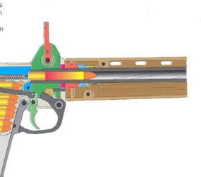
After about 3/16" (5 mm) of bolt travel (or .0013 seconds) the bullet exits the muzzle. The pressure in the barrel has now dropped to a low level.
