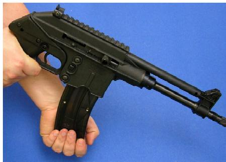
If you wish to restore the magazine in your firearm to full capacity, press the magazine catch and remove the magazine to load the missing round. Remember to keep the safety engaged and your pistol pointed in a safe direction under all conditions and always keep your finger off the trigger and outside the trigger guard until ready to fire. Never insert a live cartridge by hand into the chamber and slam the bolt closed, doing so could cause the round to discharge.
