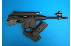
WARNING: If the recoil spring tube is not parallel with the barrel of the pistol the bolt carrier assembly is not installed correctly. Remove the carrier assembly and install it again paying close attention to the alignment of the lock tab on the recoil spring tube as you insert the carrier and also be sure that the bolt itself is always in the forward most position as you insert the carrier assembly into the receiver.
