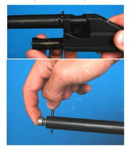
onto the recoil spring and onto the piston rod. Insert the firing pin or similar tool into the piston head hole to temporarily hold the piston head in place. While slowly pulling out the firing pin, push in the piston pin from the other side until it is flush with the piston head. Twist the recoil spring tube so that the locking tab points towards the top of the bolt carrier. Check the operation of the recoil spring by lightly pulling on the recoil spring tube to compress the spring.
