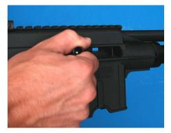
bolt stop and slowly release the operating handle, the bolt should stay open. Visually inspect the chamber to make sure it is empty. Pull back on the operating handle to release the bolt stop and release the operating handle to close the chamber. Push the remaining cartridges in the magazine forward and out.
