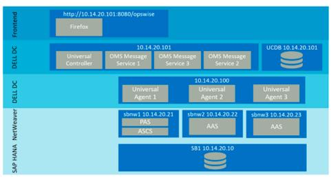
Figure 2: performance test architecture
