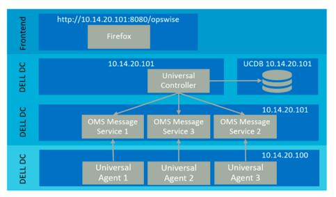
Figure 4: architecture of performance test – horizontal scalability, multiple OMS servers
