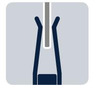
Pluggable tension-spring connection ZST
