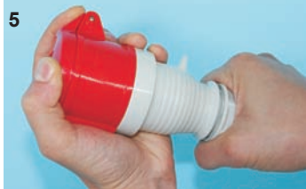
Finally tighten the cable gland (torque at least 4 Nm) - ready.
