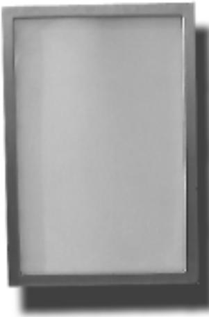
Steel Window Kits are designed for use on NEMA Type 4 and Type 12 enclosures. Stainless Steel Window Kits are suitable for NEMA type 4, Type 4X, Type 12, and Type 13 enclosures in applications where corrosion is a problem. These kits are easily installed by making a cutout in the enclosure and attaching the window and frame in place. Frames are made from heavy gauge steel and have a gray powder coat finish OR heavy gauge Type 304 stainless steel with a
