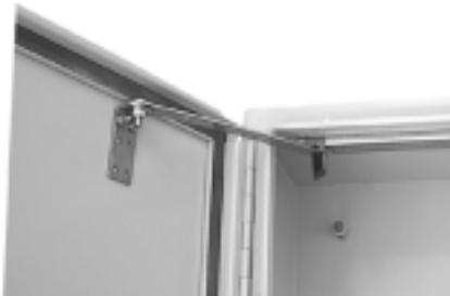
This mechanical adjustable door stop kit is designed for most standard Type 4 and 12 enclosures. It is designed for field installation, but you may order it to be installed in our shop. For proper operation, the door opening must be a minimum of 16 inches. A sliding arm with a tightening knob allows for an adjustable opening width. These kits are available in Plated Steel and 304 Stainless Steel.
