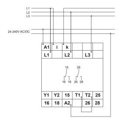
Connected 3~ with fault latch I<sub>N</sub><12A
