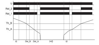
Example: I=0 Inv. with minimum monitoring (2MIN+I=0 ON) relay state invers: Rel\_1 and Rel\_2 off
