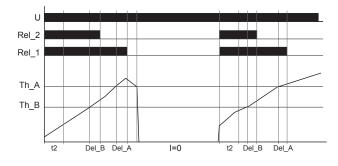
Example: I=0 Inv. with maximum monitoring (2MAX+I=0 ON) relay state invers: ReI\_1 and ReI\_2 on
