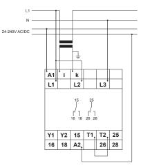
Connected 3~ with fault latch and current transformer  $I_{N}$ >12A
