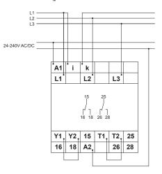
Connected 3~ with fault latch and temperature monitoring sensor  ${\rm I_N}{<}12{\rm A}$
