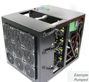
expect that electrical isolation around the cooling loop is possible because of the dielectric fluid. The pumping power required for two-phase cooling relative to single-phase cooling is reduced by about 85%, which improves system-level efficiency.
