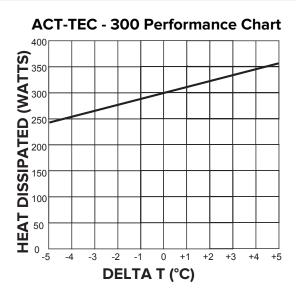
Note: Delta T is the temperature difference between the inside enclosure temperature to the outside enclosure temperature
