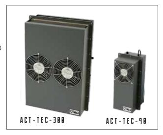
The ACT-TEC Thermoelectric Cooler series are compact solid state air conditioners. They cool the internal enclosure space with highly reliable Peltier cooling. The Peltier cooling cycle involves no moving parts, compressors, CFC refrigerants or circulating liquid. They feature a very long life as they are not vulnerable to refrigeration leaks. They exceeded the rugged industrial requirements of operating two four hours per day, seven days per week. In addition,
