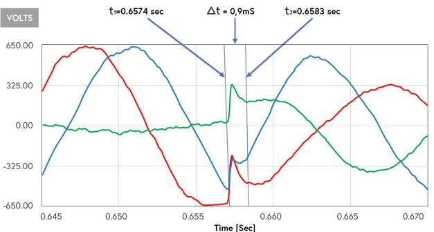
Picture shows how fast the AVE reacts to a voltage imbalance and stabilizes the system. The reaction time is less than 0.9ms.
