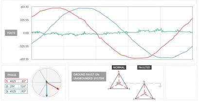
Graph shows waveform and phasor diagram for a 3-phase distribution system with ground fault on phase B with AVE deactivated.
