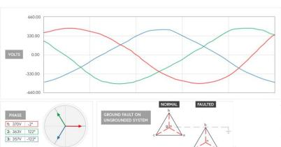
Graph shows waveform and phasor diagram for a 3-phase distribution system with ground fault on phase B when AVE is activated.
