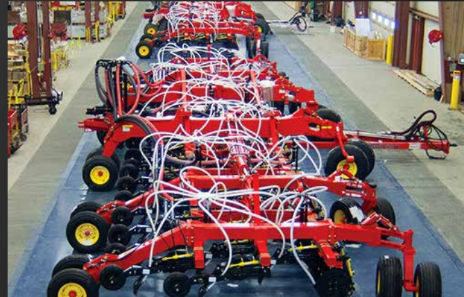
Moving Floor System – Custom Design 390' x 25' moving-floor, weighs in at just under one million lbs. and uses a string of wheeled carts, with a working surface of steel plates. 20,000 lbs. point loads; 4' per minute horizontal travel speed.
