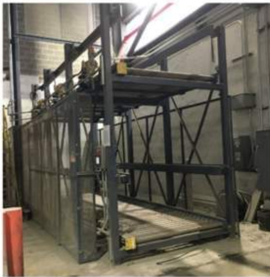
Figure 6 - WFS conveyors at tipping floor grade elevation. Example of forklift loading Tipping Floor Transfer conveyor.
