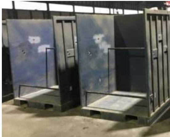
Figure 5.2.3 Example of 3-sided WFS bins
