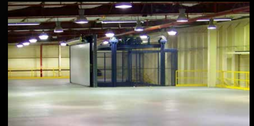
Boat Mold Lift – F Series Mechanical VRC Retrofitted design doubled storage space for fiberglass mold dollies in lamination production area. 5,000 lbs. lifting capacity.
