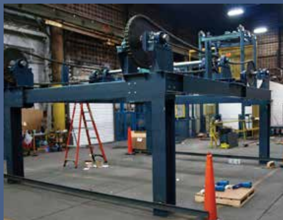
Telecommunications Lift – High-Capacity VRC Designed to move 20' shipping containers into a secure underground facility. 50,000 lbs. lifting capacity; 40' lift travel.
