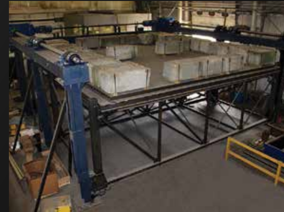
Mirror Lift System – 6-Post Mechanical VRC Winner of 2016 Governor's New Product Award. 161,000 lbs. lifting capacity; 78' lift travel; 4 levels of service; 10' per minute travel speed.
