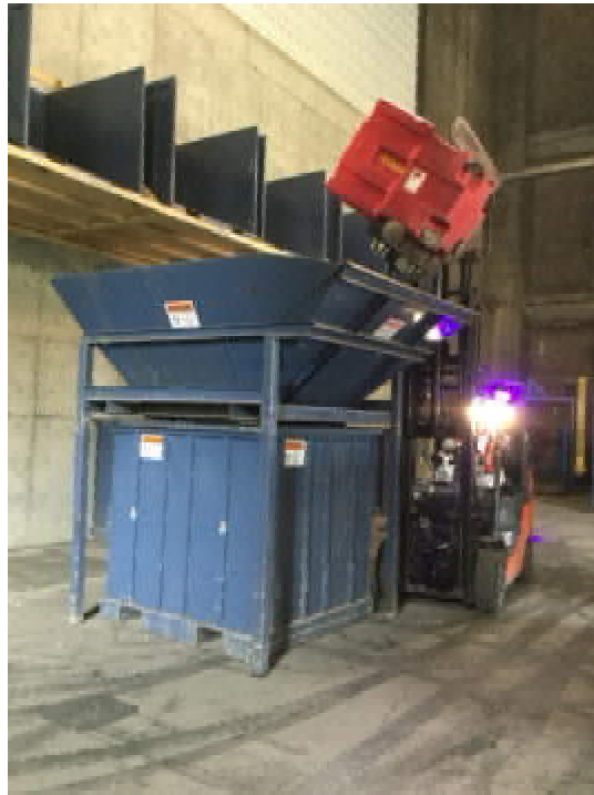
Figure 1 - Contents of the reusable totes dumped into the 4-sided fully enclosed WFS bin.
