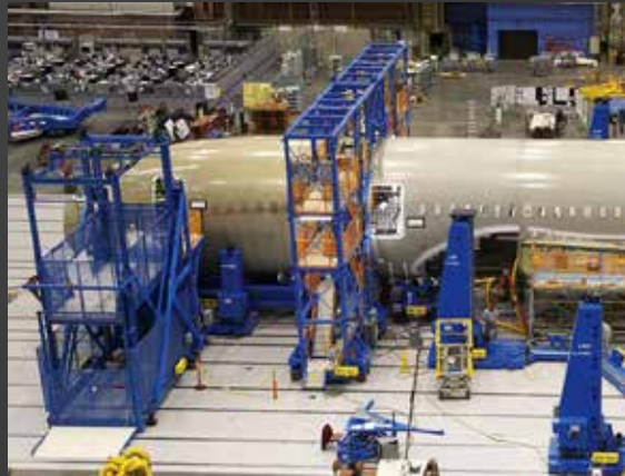
Movable Platform – Custom 4-Post VRC Includes a retractable lower aluminum ramp and power roll-up doors. 3500 lbs. capacity.
