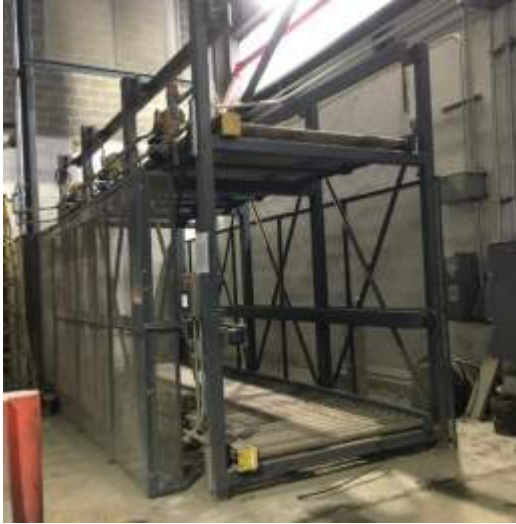
Figure 5.3.2 WFS conveyors at tipping floor grade elevation. Example of forklift loading Tipping Floor Transfer conveyor.
