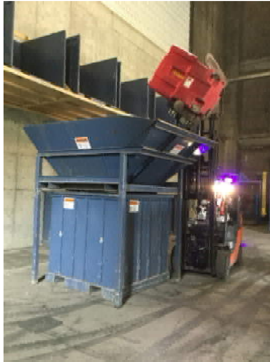
Figure 5.2.1 Contents of the reusable totes dumped into the 4-sided fully enclosed WFS bin.
