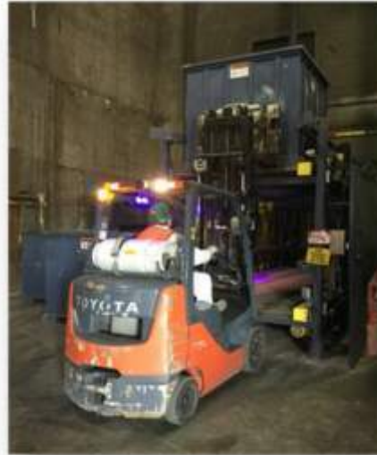
Figure 5.3.2 WFS conveyors at tipping floor grade elevation. Example of forklift loading Tipping Floor Transfer conveyor.
