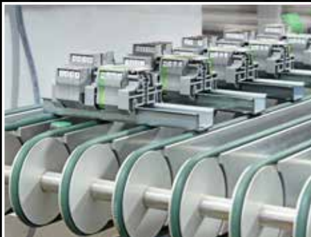
Sorting unit and buffer stores for machined terminal strips
