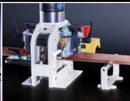
Cutting a busbar to length
