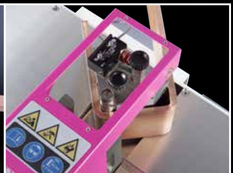
Bending a busbar
