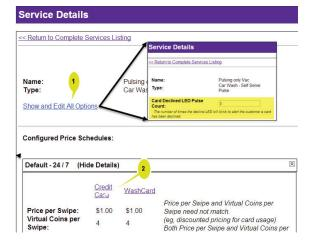
iii. Be sure to check the coin amount setting on the equipment. If it is set to \$0.25 then set the Virtual Coins to Send: at 4 per dollar; if it is set for \$1.00 then set only 1 pulse per dollar.
