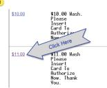
iii. 3 Order of Presentation: This determines the order in which the Price Points are assigned to the Inputs on the Terminal Controller. If the wrong amount is displayed when a button is pushed it can be corrected by changing the Order of presentation number.
