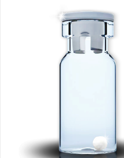
Figure 2. Schematic of small-scale resin sanitization model. This approach allowed for controlled, high-throughput testing of multiple Protein A resins, chemical sanitants, and bacterial spiking conditions.
