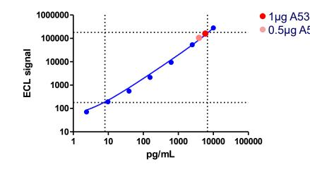
αSYN quantification assay set up: Mesoscale Discovery (MSD) 96-well assay kit was employed for quantification of total αSYN from mDAns cell lysates. Linearity test of A53T lysates (dd28) was performed with 1µg and 0.5μg of lysates from A53T mDAn. ECL signal revealed linear αSYN detection within the linear range of the calibration curve. 0.25µg/well was the condition selected for the following quantifications in mDAn cultures.
