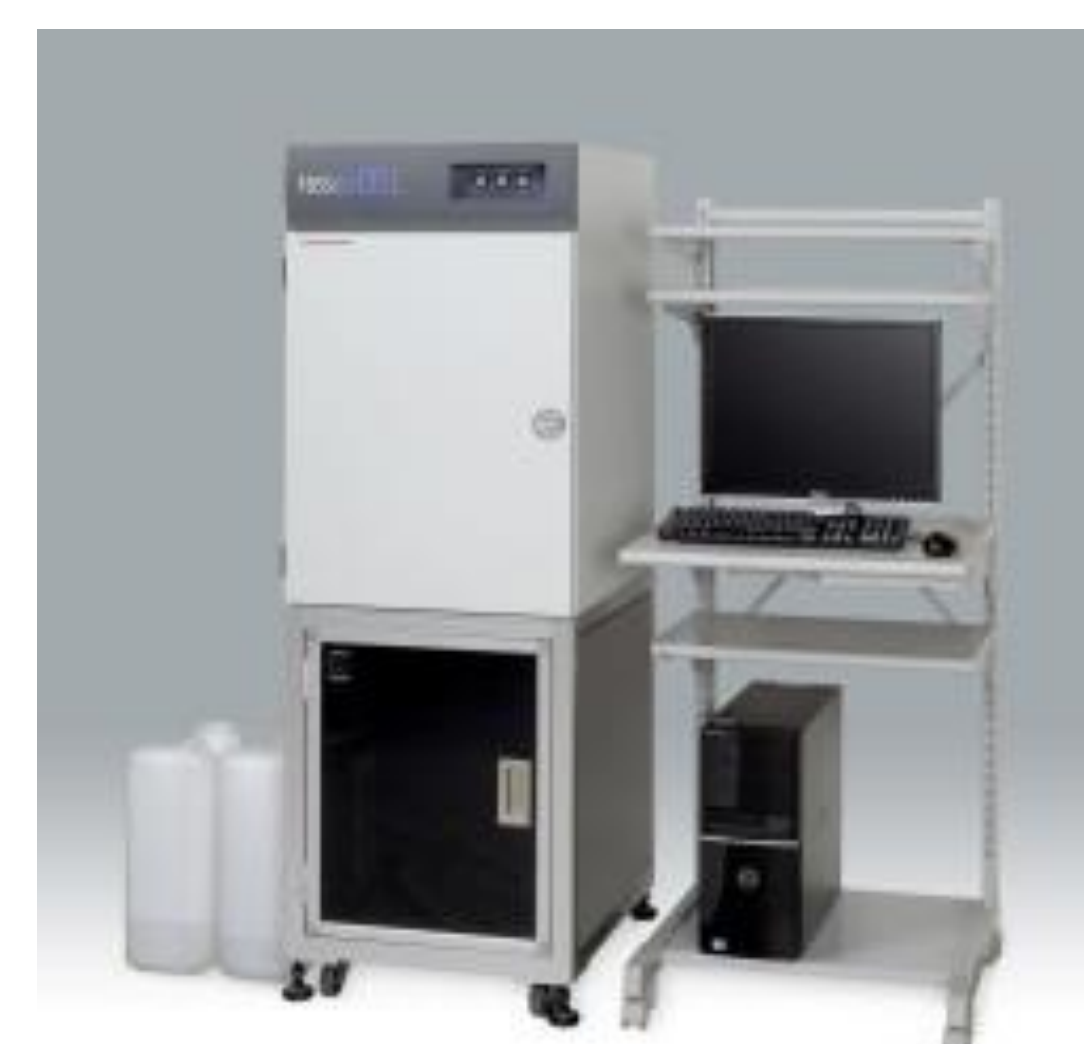
Figure 3. The Hamamatsu FDSS/μCell. Cells were treated for 14 days with drug and then Codex calcium dye was used to determine the calcium flux of the CDI cardiomyocytes.
