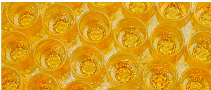
Figure 1: An example of the design of a typical MEA plate. Each well contains multiple individually embedded microelectrodes which continuously monitor the electrical behaviour of cells. Image provided by Axion Biosystems.
