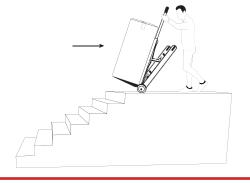
When the front of the load has cleared the edge of the landing, lean the unit forward, while holding the load in place.
