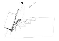
When the tracks and wheels reach the bottom landing, lean the unit forward until it is resting on the bottom of the platform.
