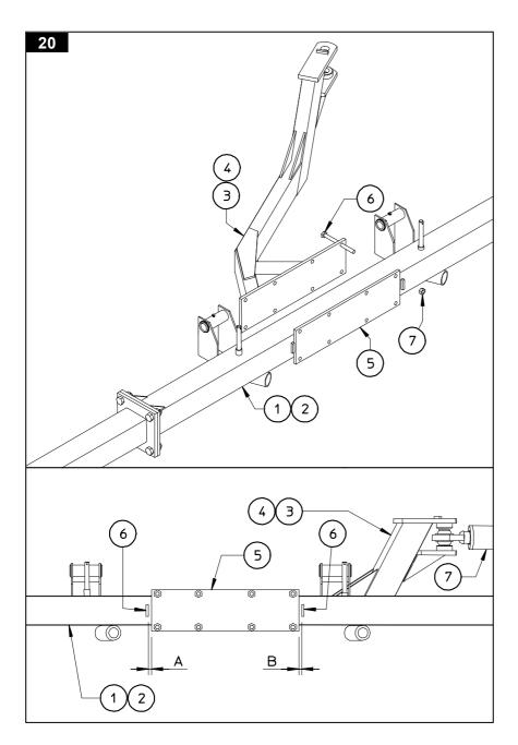
fastening them with screws 6 and nuts 7. See diagram for the correct positioning of the parts.
