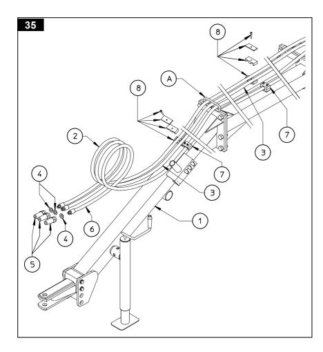
collars 9. Secure hoses 2-3-6 in the correct places with hose collars 7 and with double hose collar 8. Attach washers 4 and quick-release couplings 5 to the ends of hoses 2-3-6.
