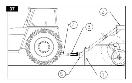
that drawbar 2 is parallel to the ground. Back the tractor up to the machine and look to see if hitch 3 is aligned with tractor hitch 4. If hitch 3 is much higher or lower than tractor hitch 4, it is necessary to change position of hitch 3 by choosing the holes in plate 5 which give the best alignment. At this point connect hitch 3 to tractor hitch 4 using a suitable pin. Next turn the parking stand crank to retract the base of the stand.
