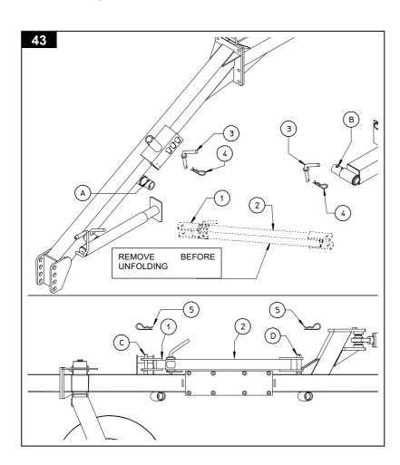
A & B and fastening them with clips 4. The transport arm assemblies are to be placed over pins C & D on the rake wheel sections as shown. Paste the transport arms to pins C & D with clips 5.
