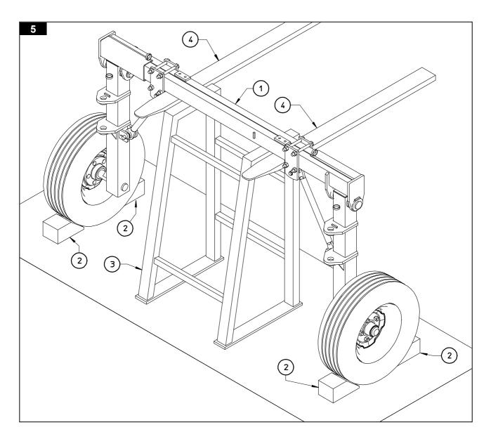
3 must be placed under the cross member. The forks 4 of a forklift may also be used to support the assembly.
