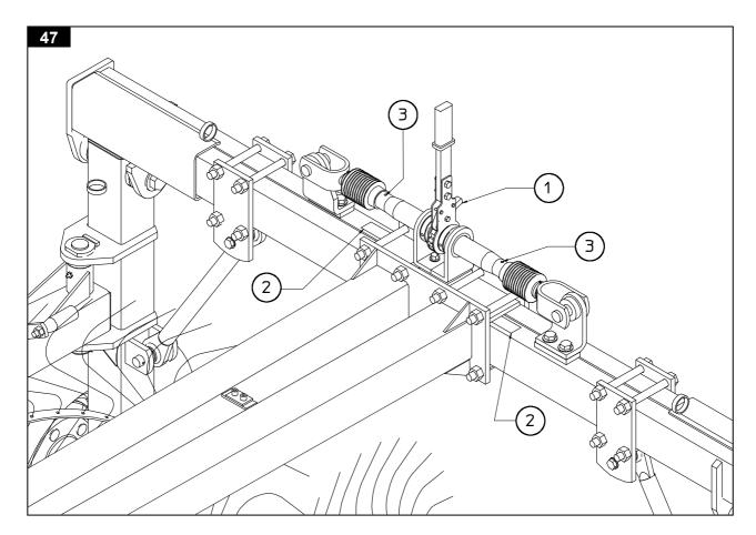
REAR OPENING STARTS AT 72" TO A MAXIMUM OF 84" AND THIS ALLOWS TO OBTAIN WINDROWS FROM APPROXIMATELY 3' AND 2" TO A MAXIMUM OF 5' AND 2".
