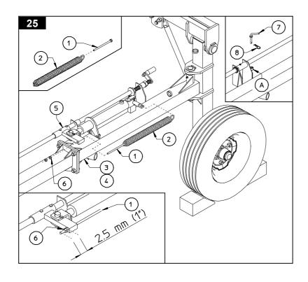
(LH - RH) and attachments 5 as shown, fastening the spring-bolt assembly in place with nuts 6. Pasten stay bolts 1 with nuts 3 so that they extend 25 mm (1") from attachment 5, as shown.
