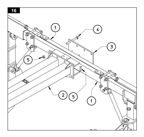
NOTE: Assemble the drawbar 2 in the middle of the cross members 1 only when the cross members 1 are pulled in together, so the drawbar 2 and counterplate 3 must be assembled between ledges 6 (see also figure 46). Attach drawbar 2 to cross member assembly 1 using counterplate 3, screws 4 and nuts 5.
