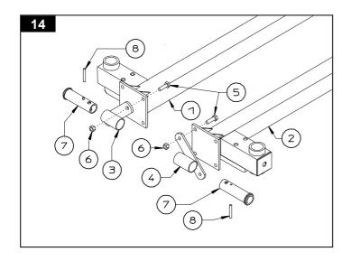
bushings 7 in the correct openings in attachments 3 & 4 (LH - RH) and fasten in place with spring pins 8.
