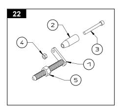
not be fully tightened, so that hand grip 2 can turn freely. Lock screw 3 in place with nut 4. Fit nut 5 onto the thread of crank 1.
