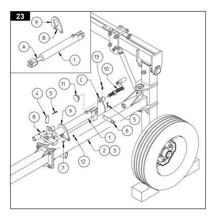
cylinder guides 9 to sections 2 & 3 (LH - RH) passing through point A and slot B. Fasten in place the cylinder guides 9 to sections 2 & 3 (LH - RH) with screws 7 and nuts 12.
