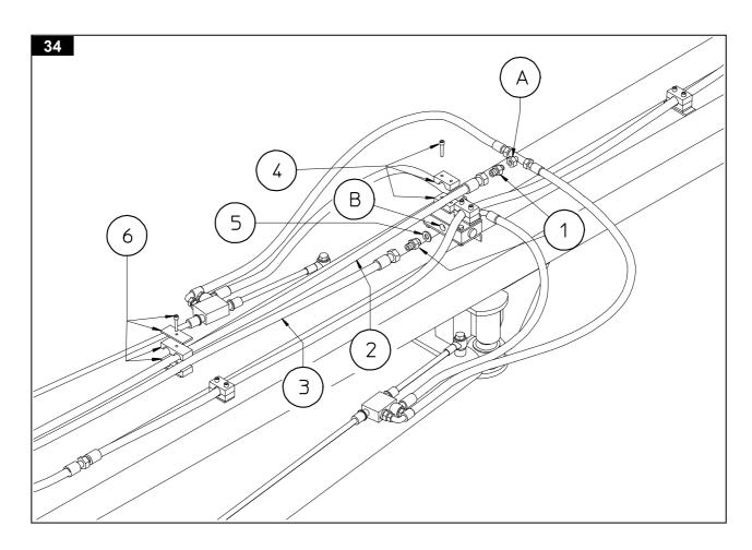
place with collars 4. Screw nipple 1 and washer 5 into hole B of the flow divider. Screw hose 3 onto nipple 1 and secure in place with hose collar 4.
