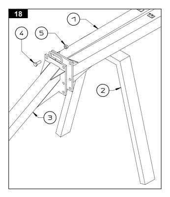
Attach the front drawbar section 3 to the center drawbar section using screws 4 and nuts 5.
