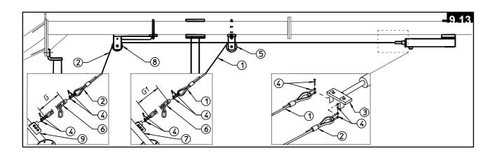
Fit cables 1-2 to cylinder 3 by using clamps 4.
