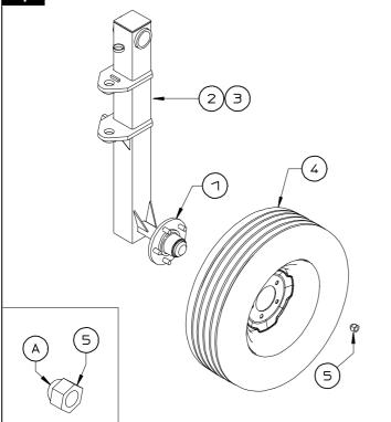
Item 5: 10 - nuts M 16 (5/8"), fine pitch and spherical cap.
