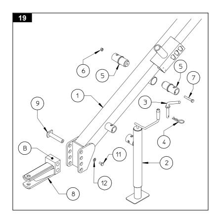
position of the parking stand is described on page 35. Insert bushings 5 in the correct holes in drawbar 1, fastening them with screw 7 and nut 6. Insert hitch 8 in the end of the drawbar and fasten with pins 9, washers 10 and nuts 11.
