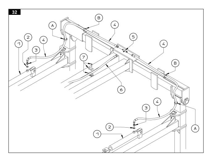
Pass hoses 4 through rings A & B and connect to T connector 5 at the center of the machine. Connect hose 6 to T connector 5 and secure in place with collars 7. NOTE: Hose 6 will also be in the next few steps.
