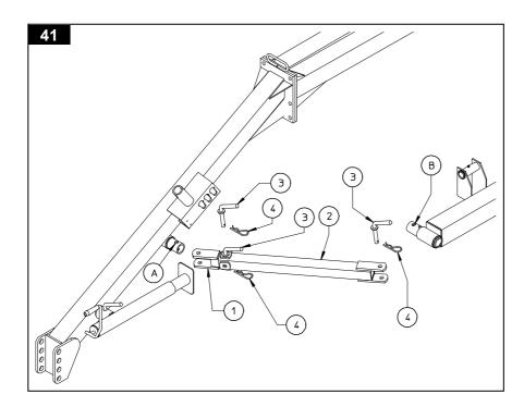
with pin 3 and clip 4. The transport arm assembly is then attached by placing the fork of arm 1 on attachment A of the drawbar and the fork of arm 2 on the rake wheel section.
