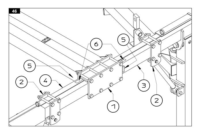
& 4 paying attention on ledges 5 welded on cross member 3 & 4. The distances must be read from label 6. The distances of cross members 3 & 4 must be the same. Once adjustments are made, fasten all screws of plates 2 and counterplate 1.
