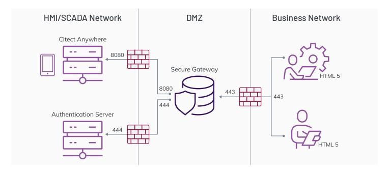
The client end runs on the Citect Anywhere Server and displays Citect SCADA graphics in the web browser. Mouse clicks, keystrokes and gestures are sent from the remote user to the Citect Anywhere Server.
