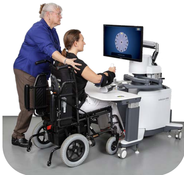
Fig 1: InMotion ARM Robotic Rehabilitation System
