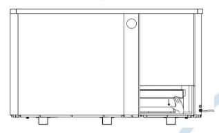
③ Fix the internal panel by two screws
