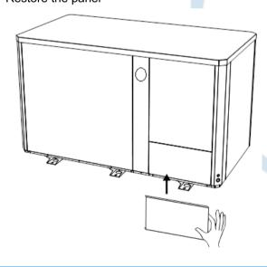
Fix the panel by three screws
