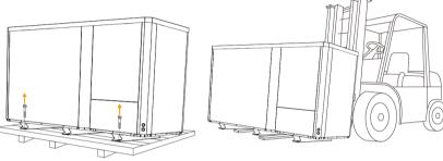
c. Do not lift by the water unions, otherwise, the titanium heat exchanger inside the heat pump may be damaged)
