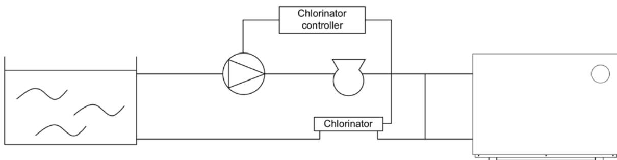
1. Chlorinator controller initiates the filtration pump.
