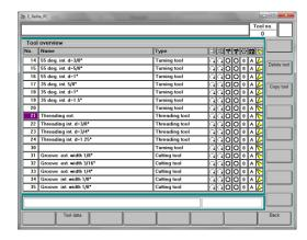
Go to Tool Overview and highlight existing Threading External Tool (21)
