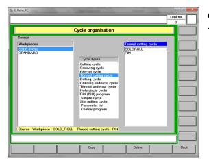
COLDROLL cycle now appears under the Thread Cutting Cycle column
