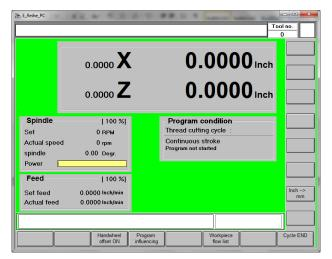
Before starting the cycle, press the Handwheel Offset ON softkey
