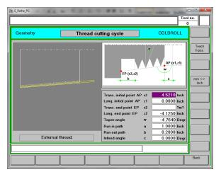
On the Thread Geometry Page, verify that the tool will clear the shoulder at the z2 value shown (-4.125 in this example).
