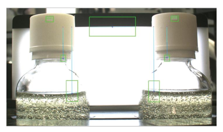
Omron's AutoVISION product inspection software checks the CBD fill level and ensures the integrity of the cap installation. The software includes thirteen vision tools that optimize common detection characteristics.
