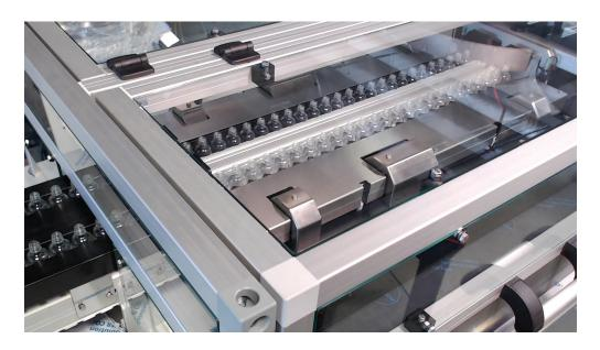
To support the requirements for ISO 5 cleanroom, several Omron D40P Series non-contact safety switches detect when filling and capping section doors have been opened.
