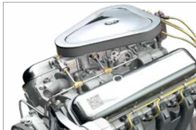
2D codes (Data Matrix) inspection on an valve cover are required for proper traceability.
