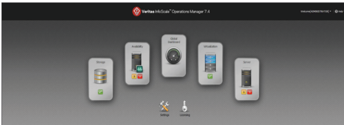
Figure 3. Admins can use InfoScale's central dashboard, Operations Manager, to manage data and application failures.
