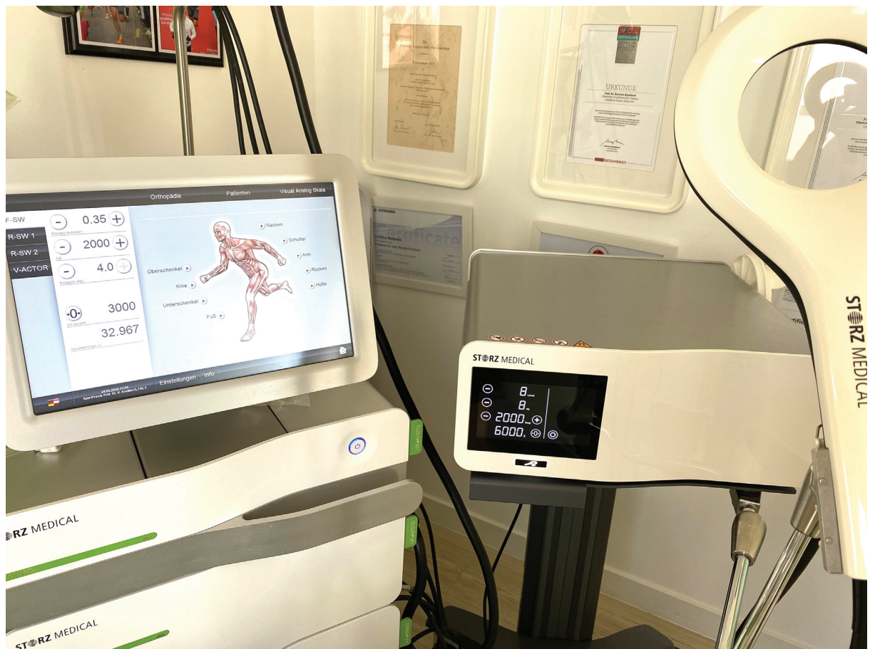
Figure 4. High-energy focused electromagnetic extracorporeal shockwave therapy (ESWT, Storz Ultra by Storz Medical, Tägerwilien, Switzerland, on the left) and novel extracorporeal magnetotransduction therapy with Magnetolith (Storz Medical, Tägerwilien, Switzerland, on the right) for bone stimulation therapy in scaphoid nonunion.
