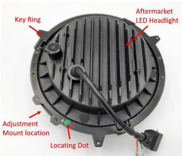
**Step 1:** Take the Key Ring and align the three keyways and keys of the LED headlight. The LED headlight should be facing up and the adjustment mount location to be positioned to the bottom left. A colored locating dot should be visible.
