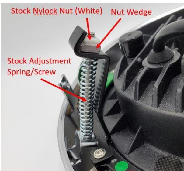
**Step 6:** Now add the stock adjustment spring between the bezel adjustment mount and the Adjustment piece. Try to align the spring with both holes. *Take caution, the spring may launch under load.*
