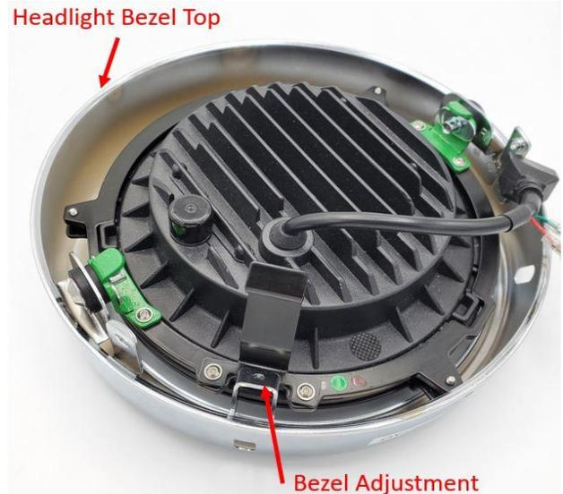
**Step 4:** Add the side mounts to the key ring using the supplied M3 x 5 screws. Do this for both side mounts. Both side mounts are identical. Now add the Adjustment piece as shown using the M3 x 5 screws.
