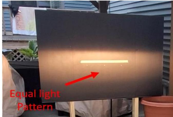
**Adjustment:** After the headlight is installed on your bike position the bike 10 feet from a blank wall. Measure from the ground the height of the headlight (to center) with the rider sitting on it. Now mark your wall with this dimension. Adjust the headlight until the low beam pattern is equally spaced over the line on the wall.
