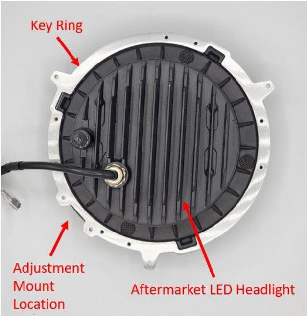
**Step 1:** Take the Key Ring and align the three keyways and keys of the LED Headlight. The LED headlight should be facing up and the adjustment mount location to be positioned to the bottom left.
