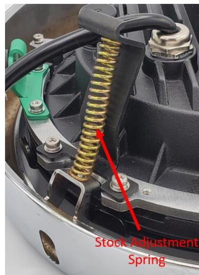
**Step 7:** Now add the stock adjustment spring between the bezel adjustment mount and the adjustment piece. Try to align the spring with both holes for the next step. *Take caution, the spring may launch under load.*
