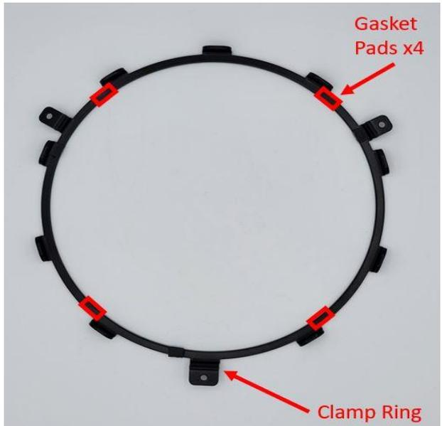
**Step 2:** Apply the 4 provided EPDM gasket cutouts to the bottom side (tabs facing up) of the clamp ring in the approximate locations described above. This will cushion the LED headlight in the setup and reduce vibration. When applying use pressure for 20 seconds. This is an optional step.
