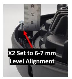
Level Adjustment: On the Stryker Bezel set the M4 screw (X2) to a distance of 6-7 mm from the top of the adjustment piece. This should give the headlight assembly a centered adjustment. This will differ on the Raider Bezel. On the Raider set the top adjustment to around 10-11 mm and the bottom adjustment to 6-7 mm.
