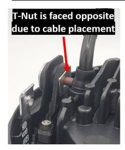
**T-Nut Placement:** You may come across LED Headlights with a wire placement very close to the side mounts. If this is the case flip the T-Nut so that it goes inside the Side mount hole. This will open up clearance between the LED adapter assembly and the LED cable.
