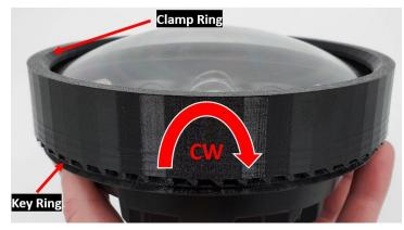
**Step 2:** Holding the LED Headlight lens up and keeping the Key Ring flush with the headlight apply the Clamp Ring. Spin the Clamp Ring clockwise. The threads should engage the Key Ring. Tighten the Clamp Ring (DO NOT OVER TIGHTEN). The Clamp Ring should be tight enough where the headlight has no play within the setup.
