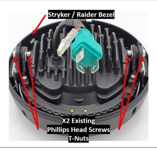
**Step 5:** Slide the Yamaha Stryker / Raider Bezel over the top of the LED bracket. Line up the side mount holes with the bezel mounts. Use the existing hardware from the stock headlight. Have the T-Nuts facing each other.
