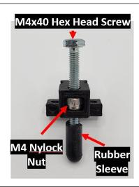
**Step 6:** Build the Adjustment setup (X2) using the M4x40 Hex head screw, the M4 Nylock Nut and the rubber sleeve. Make sure the flat portion of the nut is facing up toward the Hex head. This assembly may be built for you. The nut may be adhered in the adjustment mount.
