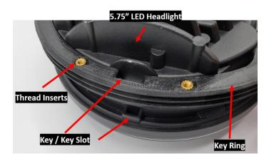
**Step 1:** Take the Key Ring and align the keyway and key of the LED Headlight. Make sure the thread inserts are facing away from the headlight. Also be sure to have the key ring sit flush with the headlight.
