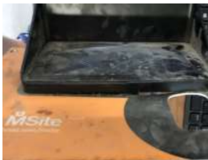
Dented front plate and cracked screen
