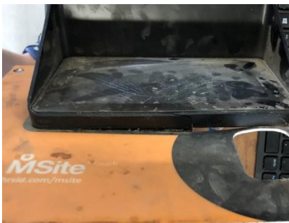
Dented front plate and cracked screen
