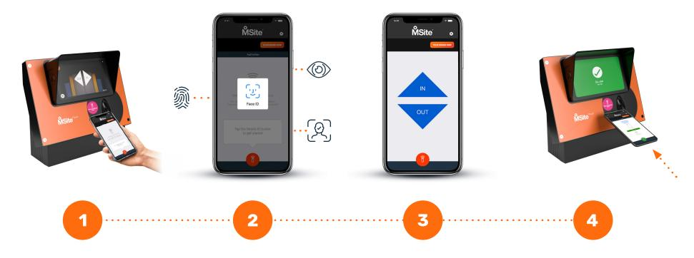
Open the MSite Workforce App & hold near fingerprint reader, **pressing the red button** (no need to hold)
