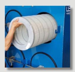
The simple and secure design is widely considered as the best in the industry. Using stainless steel brackets, cross rod and a cast aluminum handle, it will stand up to the toughest environments, both outside and inside your facility. There are no knobs to turn, no moving rails, no interior yokes or threads to catch, or holes to center up — just drop in the door and clamp down. Lift the handle and you're holding the best door the industry has ever seen.
