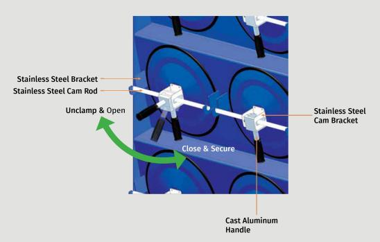
Only aluminum and stainless steel parts are used in the construction of the door cam and mounting brackets for maximum durability in any environment. Simply set the door in place and pull the handle down to lock the cam.
