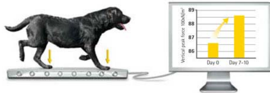
Biomechanical force platform with integrated balance. Speed between 1.7 and 2.1 m/s
