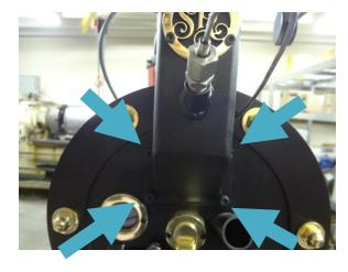
Then replace feed hopper back on the front of the face plate of the roaster using a 5/32 Allen wrench.
