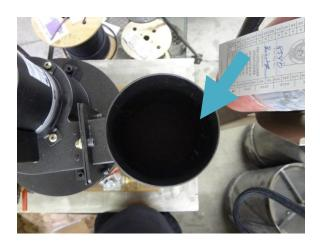
Clean the inside of the hot air exhaust vent with a vacuum or a wet wash cloth use soap and water.
