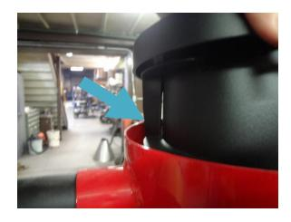
Put black lid back on and make sure the pieces look like this in order to put it correctly back on the chaff cyclone. The arrow is pointing to show the inside of the lid to be matched up with the feed hopper pipe.
