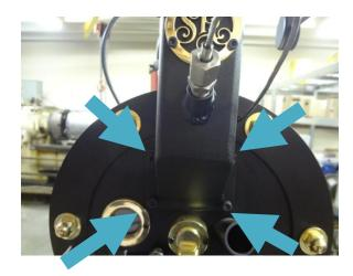
Go to the front or face of the roaster there are 4 black cap screws for the feed hopper use a 5/32 Allen wrench to remove them. After they are off the roaster carefully pull the front of feed hopper off. The feed hopper pipe will come off with it.
