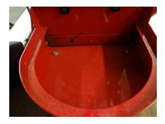
Wipe clean under the cooling tray with soap and water. Pull handle forward and clean where the flap comes down. Arrow is pointing to flap.
