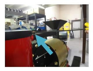
Using a 3/16<sup>th</sup> Allen wrench remove the 3 black cap screws and washers. (Picture is shown with fan removed)
