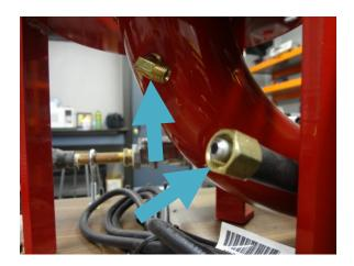
Remove hose with a 13mm wrench, pliers, or a crescent wrench. Wipe down the inside of both the hose and elbow.
