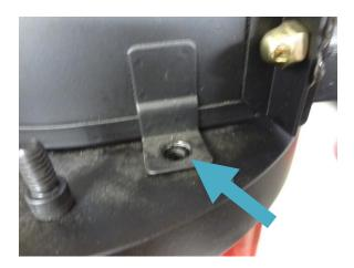
One of the black cap screws removed from the bottom of the fan.
