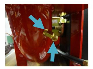
Elbow should be tight and facing the hose. Threads on elbow will not be completely inside the roaster.
