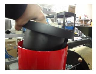
Remove black lid by lifting up if you can lift up with both hands. You can wipe down all of the lid and around the inside with soap and water.
