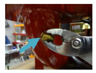
After cleaning, place elbow back in the hole using the crescent wrench or pliers by turning the elbow to the right.
