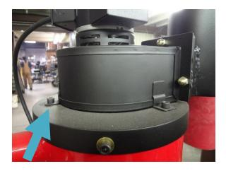
Next step is to remove the fan from the top of your chaff cyclone. Remove the 3 black cap screws with a  $3/16^{th}$  Allen wrench. Be careful that the fan doesn't fall off the roaster.
