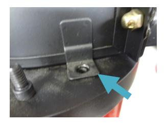
Be sure all 3 holes are matching and then loosely screw black cap screws in using a 3/16<sup>th</sup> Allen wrench. Once all 3 are loosely in the holes tighten them before moving on to next step.
