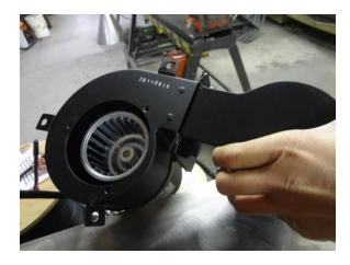
When setting the roaster fan down be sure it's on an even flat surface. Check to see if fan needs to be wiped down, if so lightly use a damp wash cloth. Be careful of your fingers.
