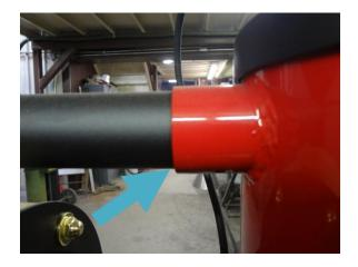
Be sure feed hopper pipe is in with the chaff cyclone. End of feed hopper pipe should fit snuggly into the chaff cyclone.
