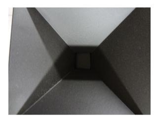
Clean inside of feed hopper before replacing back on the front of the roaster. Clean with a wash cloth using soap and water. Be sure to get all of the soap out since this is where you place your coffee beans to be roasted.
