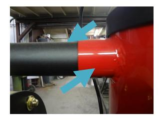
Feed hopper pipe should now be unattached clean the inside of the pipe (arrow is pointing to the pipe) with soap and water and also the inside of the chaff cyclone (arrow pointing).
