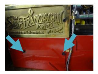
Remove side door by taking off the two black cap screws with a 5/32 Allen wrench.
