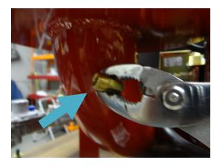
Using a crescent wrench or pliers turn elbow to the left should be on there tight in order to clean elbow.
