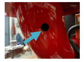
Clean the end of the elbow and the hole from where the elbow came from. Just wipe down with a wash cloth and soap and water. Put part of your cleaning wash cloth inside the hole where you just removed the elbow from and turn clock wise to clean inside it.
