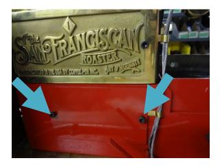
Wipe completely dry when finished and place the door back on the roaster using the 5/32 Allen wrench to put back the 2 black cap screws. Be careful to not get the air and bean probes caught in the door. Make sure both black cap screws are tightly back in place but not too tight.
