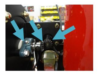
Remove black cover where the motor is with a 3/16<sup>th</sup> Allen wrench only the top two black cap screws, and grease the gears with any kind of high temp bearing grease (arrows pointing to gears and bearing). Replace black cover and 2 black cap screws at the top with a 3/16<sup>th</sup> Allen wrench. Using a grease gun put one to two pumps of grease in the bearing fitting.
