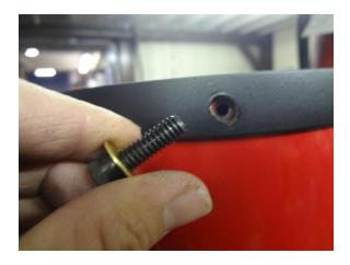
When putting back on the black cap screws remember the brass washers. Use a  $3/16^{th}$  Allen wrench to put all 3 black cap screws and washers back on.
