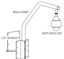
Fig. 4: Roof mount (IP66)
