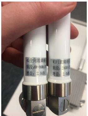
9. Connect the 4G antenna to the marked 'LTE' port on the side of the gateway by pushing and then screwing it into place, ensuring it is screwed on firmly and straight. **This must be done before powering on the gateway.**
