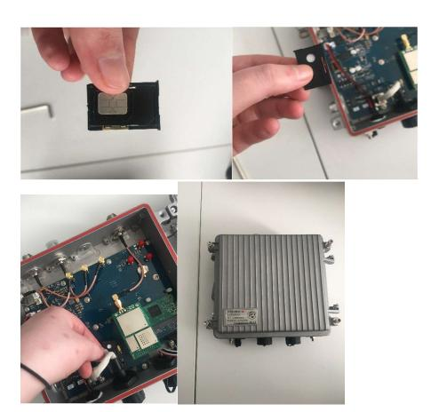
7. Connect the long LoRa antenna to the marked 'LoRa' port on the top of gateway by pushing and then screwing it into place, ensuring it is screwed on firmly and straight. **This must be done before powering on the gateway.**
