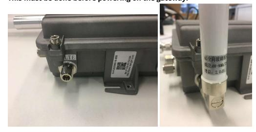
10. Connect the WiFi antenna to the marked 'WiFi' port on the top of the gateway by pushing and then screwing it into place, ensuring it is screwed on firmly and straight. **This must be done before powering on the gateway.**
