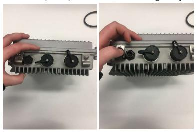
14. Push the end of the power cable into the power port of the gateway and screw into place.
