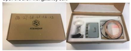
2. Remove the gateway device, the LoRa and and WiFi antennas, and the box containing the PoE connector and kettle plug. Unless otherwise specified, the remaining items in the gateway box can be ignored.
