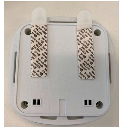
Figure 2: AQ+ device fixtures
