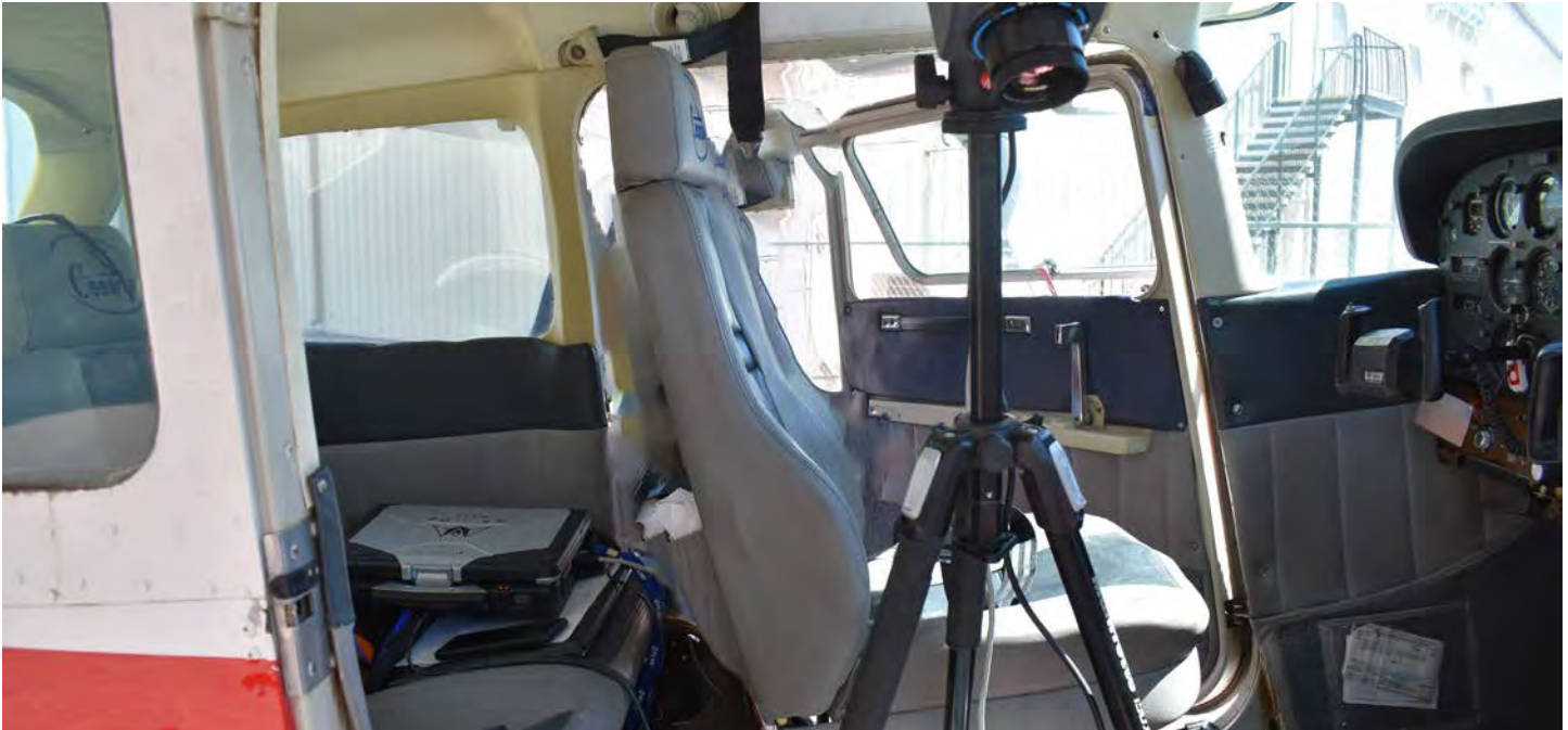
FLIR infrared camera mounted to tripod in cabin. Must be secured by multiple ratchet straps of equivalent.
