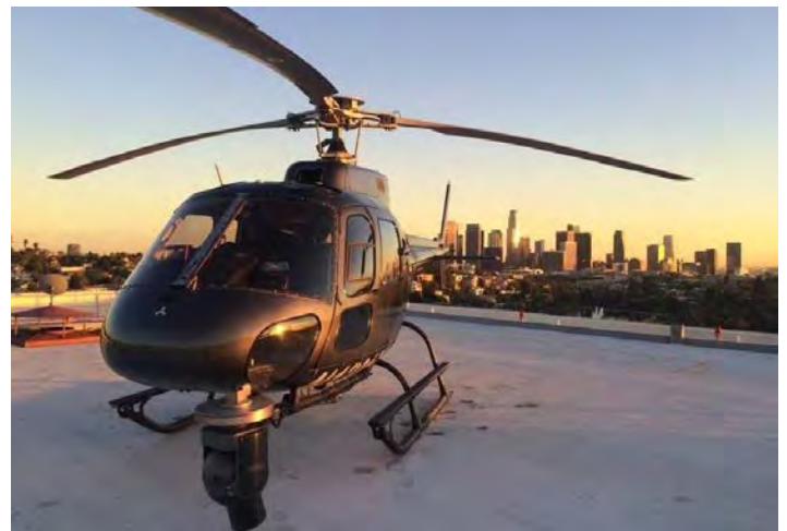
Example of a helicopter with nose-mounted camera gimbal. Source: orbicair.com
