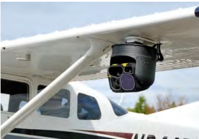
Wing-mounted gimbal on Cessna. Source: soloy.com
