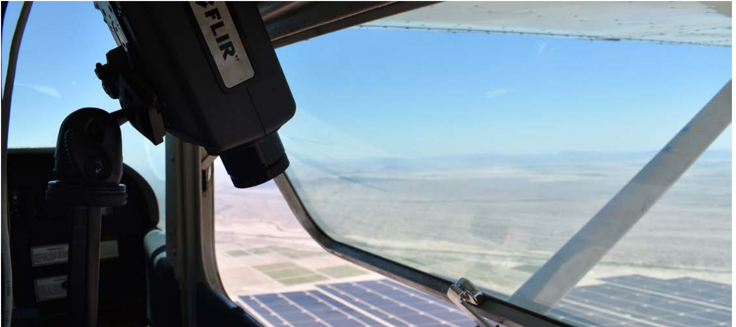
Open window on Cessna 172 with thermal camera pointing downward.
