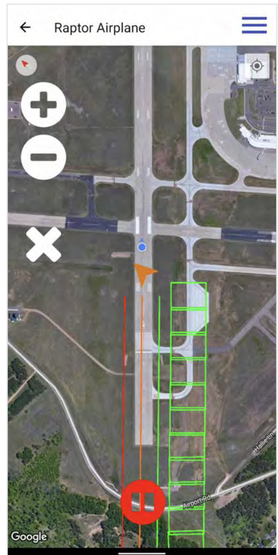
Raptor Maps coverage application for manned aircraft. Green boxes indicate coverage, blue arrow indicates aircraft direction, orange chevron indicates north.
