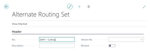
After that, you can add all those machine and/or work centers to the alternate routing set that can work as alternative resources within one routing.
