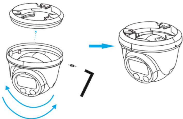
**Note:** A small “lip” is present on the inside of the base. Secure the interlocking ridges underneath this lip before attempting to snap into place.
