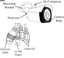
**NOTE:** Screw in the antenna into the antenna jack before installation.
