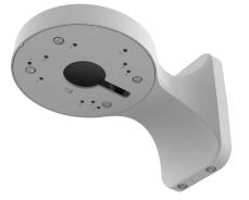
This ClareVision Wall Bracket can be used with all ClareVision Fixed Lens Dome camera to help manage cables and protect terminations at the camera installation locations. The wall bracket can be easily installed on indoor and outdoor walls, keeping the dome camera pointed down towards the ground to minimize rain impact on the dome cover and protect image quality.
