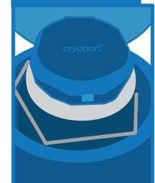
Close the hinged cap by pulling down on the lid. Let the shipper stabilize, undisturbed, overnight.
