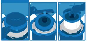
Open the hinged cap by pulling up on one of the two lift handles on the lid. With gloved hands, pull up on the circular handle in the center of the vapor plug to remove the vapor plug. Set the vapor plug aside.
