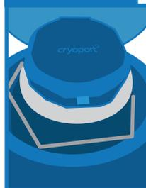
Close the hinged cap by pulling down on the lid. Let the Dry Shipper stabilize, undisturbed, for at least 30 minutes before handing it over to the carrier.
