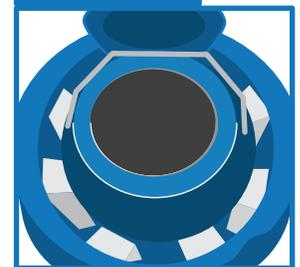
Slowly pour Liquid Nitrogen into opening. (Cryoport Client Care will provide information on the amount of LN2 to use for your specific use case.)
